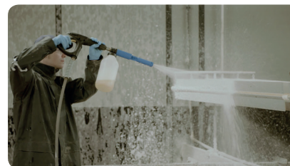
STEP 2 Apply foam with high pressure foam lance (50-150 bar).
