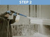
Apply foam with high pressure foam lance (50-150 bar).
