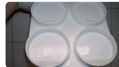
STEP 3 Pour the excess of milk away by turning the testplate until the milk reaches the marks on the testplate.
