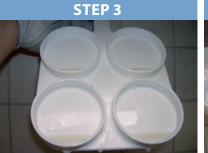
Pour the excess of milk away by turning the testplate until the milk reaches the marks on the testplate.
