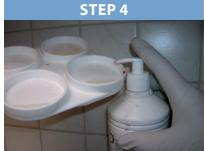
Add to each cup 2 ml Keno<sup>®</sup>test, and mix the solution during 10 seconds.
