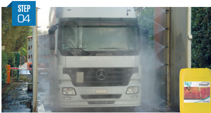
STEP 04 Disinfect (spray or foam) Disinfect all surfaces inside and out with the right disinfectant. Work your way down from the top to the bottom and pay attention to cracks and wheels. Do not forget the underside of the vehicle. Dilution: 0.25 - 0.5%.
